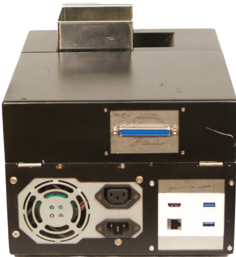
▲ Graham has ensured that Raspberry Pi's modern ports are accessible from the back of the unit
