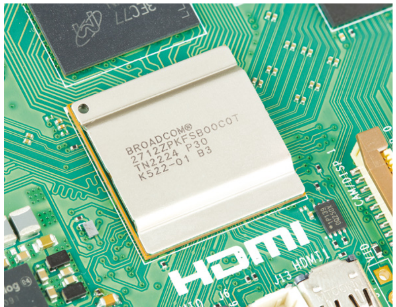
◀ The path between Raspberry Pi 5's BCM2712 and RP1 ▼ Raspberry Pi 5's BCM2712 system-on-chip
