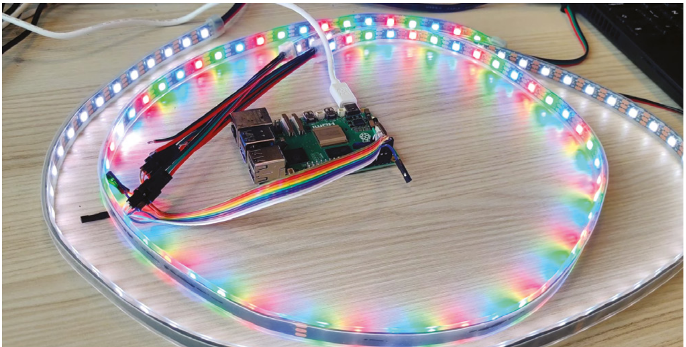
▲ WS2812 LEDs being driven by a Raspberry Pi 5
