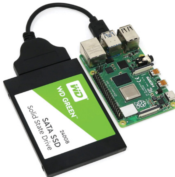
Left ■ Connect a spare 2.5-inch SATA SSD to Raspberry Pi with this adapter cable
