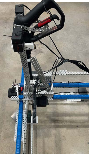
▲ The APC pulls the trigger on the pressure washer wand in a very simple solution to activating it
